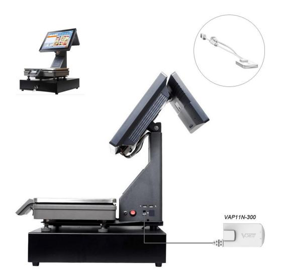
2. The power supply voltage of VAP11N-300 is DC5V-15V, input power is not less than 2.5W, if the USB interface of the electronic scale can meet this requirement, the bridge can be powered, or you can use other ways to power the bridge. (DC supply and USB can not be powered at the same time)
